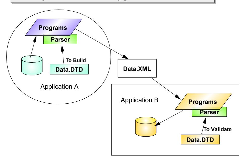
In this example, two different applications utilize XML. The programs use the DTD to ensure the XML document format created in the first program and sent to the second program meets the specifications for that data exchange.
