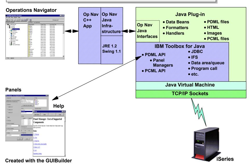
This picture shows the ToolBox and its capabilities that support both the creation of GUIs using the GUI Builder and the run time environment.
