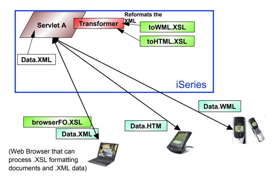
This example shows the use of a common XML document used by a variety of devices. This is accomplished by using XSL and the transformer.
