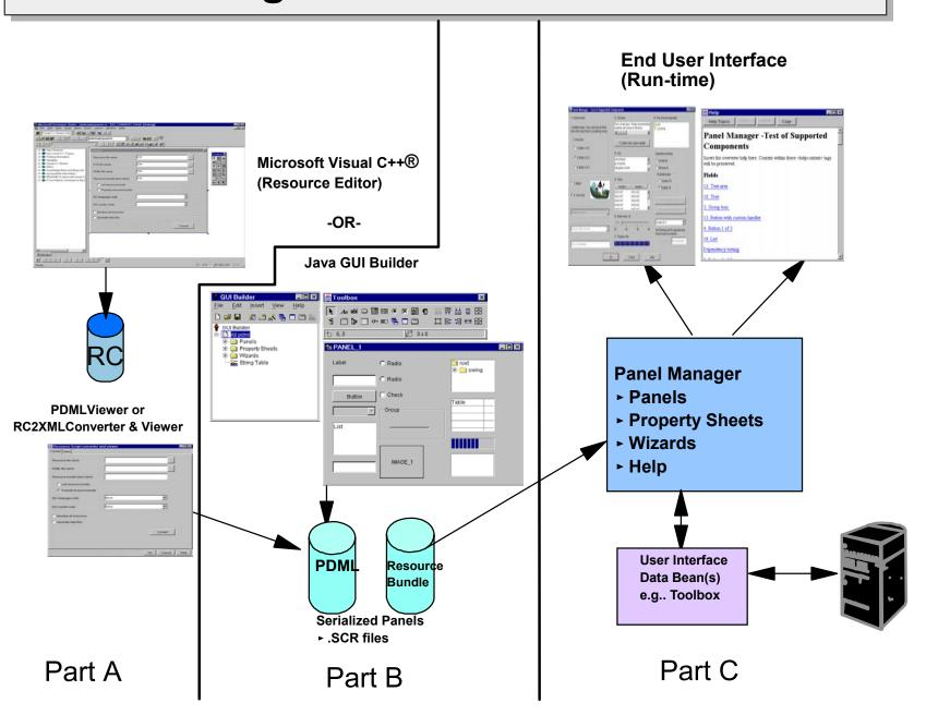
This picture shows how an existing Visual C++ display and a Java GUI can be turned into XML.
