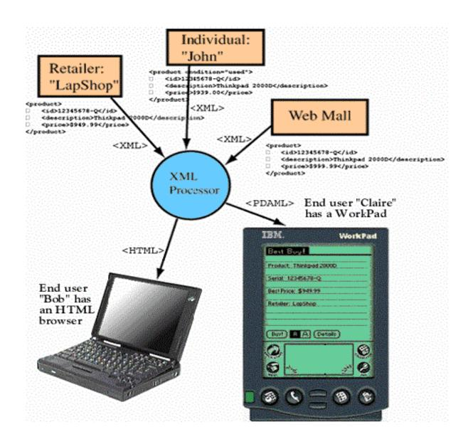
This picture is a summary of all the components required for an XML implementation... XML, a parser, XSL, stylesheets, DTDs and the device protocols to use... But once implemented, this picture shows the tremendous flexibility available with XML in reusing data created once for a variety of users in a variety of formats.
