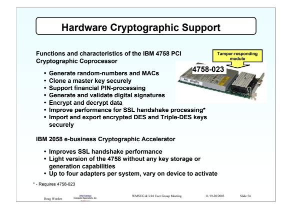
The 4758 PCI Cryptographic Coprocessor provides cryptographic processing capability and secure storage of cryptographic keys.
