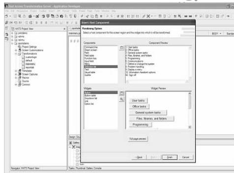
HATS Studio is a plug-in to the Eclipse-based WebSphere Studio Development Tools. It provides an easy-to-use wizard-based environment for converting host screens to a web-like appearance and functionality
